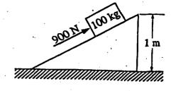
. A constant force of 900 N pushes a 100 kg mass up the inclined plane shown above at a uniform speed of 4 m/s. The power developed by the 900 N force is most nearly
