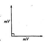
A stationary object explodes, breaking into three pieces of masses m, m, and 3m. The two pieces of mass m move off at right angles to each other with the same magnitude of momentum mV, as shown in the diagram above. What are the magnitude and direction of the velocity of the piece having mass 3m?
